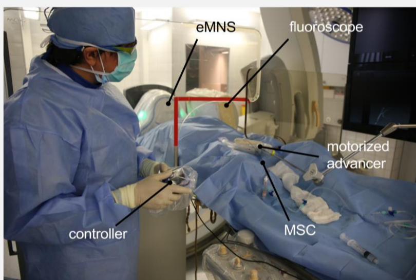
Figure 1. Remote control of the MSC with a joystick controller and fluoroscopic feedback. The catheter is navigated with the magnetic field generated by the eMNS and advanced/retracted with a motorized advancer.
